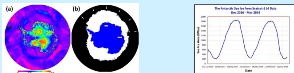
Figure 2 : An example of (a) False Color Image of Scatsat-1 Scatterometer data over the Antarctic for September 25, 2020, (b) corresponding sea ice image (sea ice is white, Antarctica is masked out and (c) The Antarctic Sea Ice Derived using Scatsat-1 Data (L4 Product at 2.25km).
