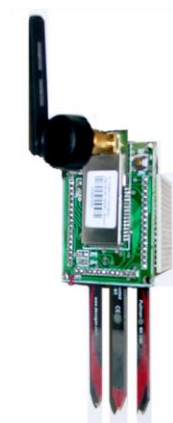
Fig. 3: Sensor Node designed at PRL (Mass : ~50 gms)
