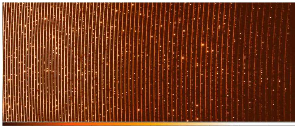
Fig 4. The Star spectra and ThAr calibration spectra recorded simultaneously for precision radial velocity measurements. The continuous lines with absorption features is the star spectra coming from the star fiber and the bright dots represent the Thorium-Argon spectra. Each line represents one Echelle order and the orders ran from 162 (3700Å) to order 72 (8500Å).
