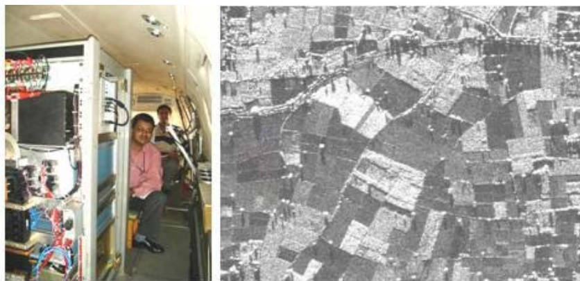
Fig.-4 : DMSAR System Mounted in Beechcraft and a Sample of High Resolution Imagery Obtained by DMSAR
