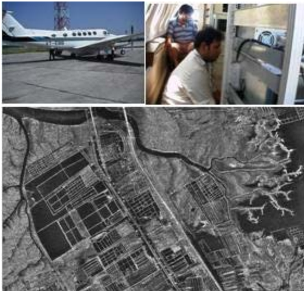
Fig.-2 : ASAR System Mounted in Beechcraft and a Sample of Imagery Obtained by ASAR
